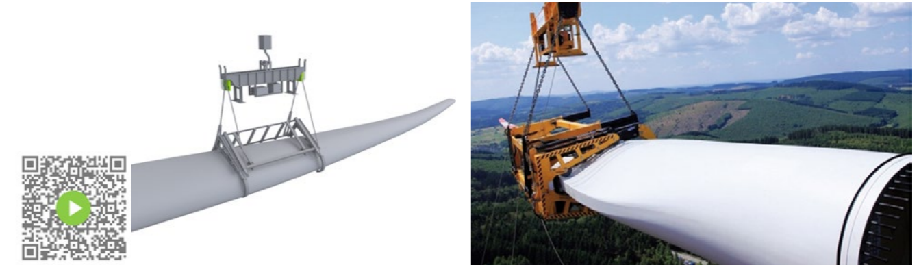
Blade Turning Device Transporting bulky, sensitive rotor blades
